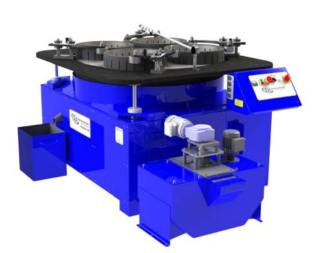
The Lapmaster Model 48 is equipped with a 48 inch (1219mm) diameter lap plate. This is manufactured from Grade 300 grey cast iron to ISO 185(2005). It consists of individual segments bolted to a support plate.
